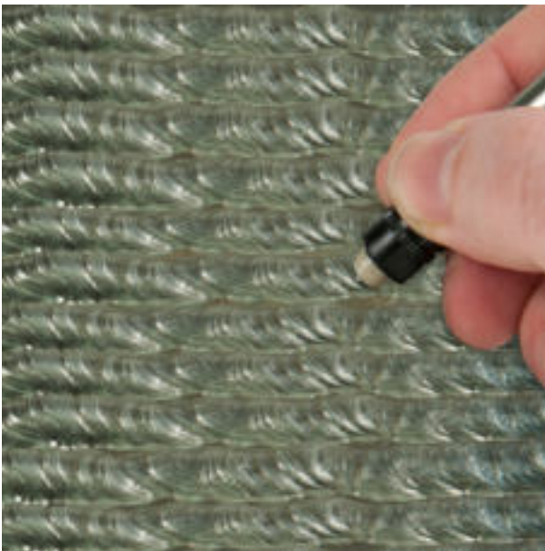
Fig.1: Measurement of a cladding coating using the FGB2 probe. The probe was placed at an angle for better visibility only; during actual operation, it must be held perpendicular to the surface.
