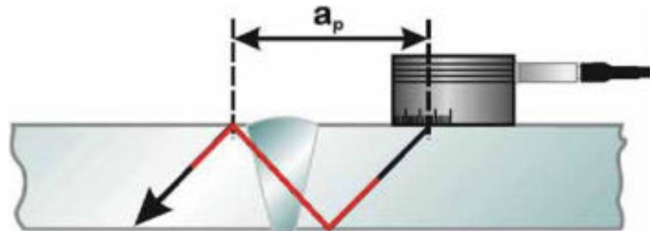
Automatic monitor positioning according to the selected skip distances
