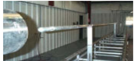
Drilled “drill collar” with mandrel for centric internal measurement with differential probe – static HotSpot procedure
