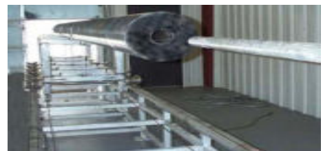
Drilled “drill collar” with mandrel for centric internal measurement with differential probe – static HotSpot procedure
