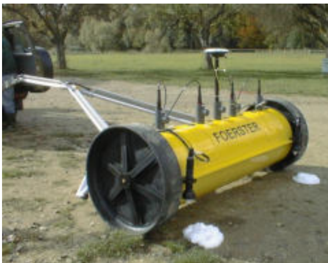
FOERSTER MULTICAT, view onto the foam marking system
