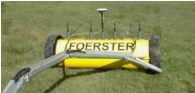
FOERSTER MULTICAT equipped with 4 FEREX probes and GPS antenna
