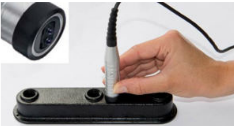
Fig.2: Measuring lacquer on a rough surface with the V7FKB4 probe
