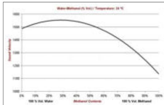
The interdependency of concentration and sound velocity using the example of the mixture Methanol and water
